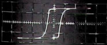
DISPLAY OF INTEGRATED WAVEFORM —transformer secondary voltage integrated and plotted against the transformer primary current—for enabling study of B-H loops of transformer cores.
