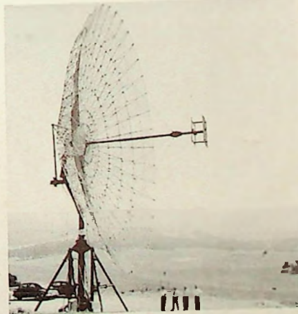
Wednesday afternoon will find field trippers in the pleasant countryside examining this 60-ft dish, first to contact Sputnik I by radar, and other structures at the SRI/Stanford field sites
