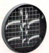
This oscilloscope display shows the output from a commercial transducer (upper trace) and the output from a developmental transducer (lower trace)—simultaneously.
