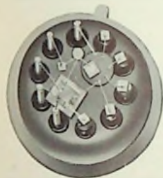
Typical example of multichip circuits: General Instrument NAND-Gate on TO-5 header
