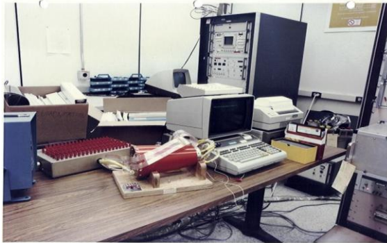
Guidance section under test with HP controller, Video Monitor Printer, Floppy disk software , breakout box, Ionizer and test cabling.
