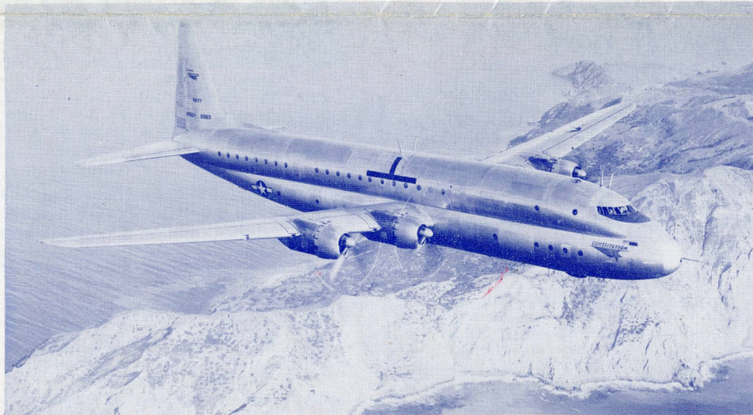
The Navy's largest airplane, the CONSTITUTION, with two complete decks connected by spiral staircases—wing span 189 feet, length 156 feet, powered with four Pratt and Whitney engines totaling 12,000 horsepower
