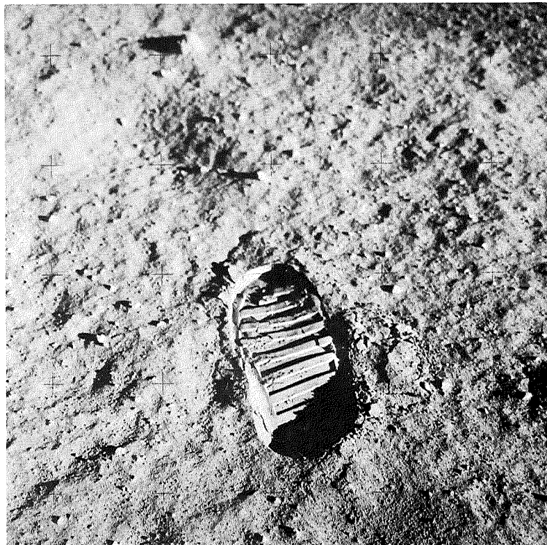
FIGURE 1-27.—The astronaut photographed his own footprint to permit later study of the lunar surface bearing strength. The thin, crusty appearance of the surface was similar to that discovered during the Surveyor soil mechanics experiments. (NASA AS11-40-5877)
