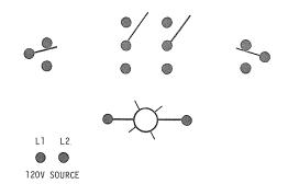
Connect the components shown so that the lamp may be turned on and off from each switch location regardless of the relative position of the other switches.
