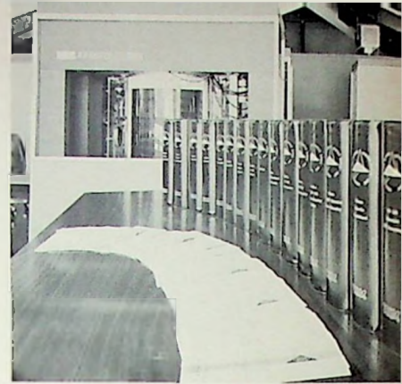
In processing center at Squaw Valley, Ramac 305 has all these volumes of detailed programming and scoring procedures committed to memory
