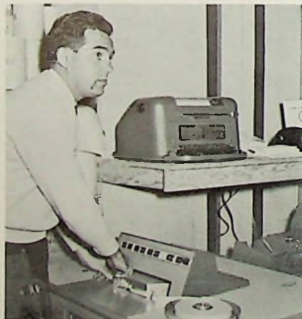
T. C. Bailey of IBM, San Jose, developed the punch-tape recorder shown. It was part of the system which produced scoring results within 1 minute of event
