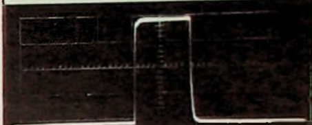
UNRETOUCHED PHOTO OF OUTPUT PULSE, MODEL L2005 (Horizontal scale: 5 μsec/cm)
