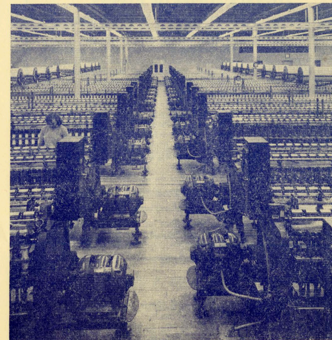
Twisting Frames with Individual Textile Motor Drives in the Cotton Industry in the South
