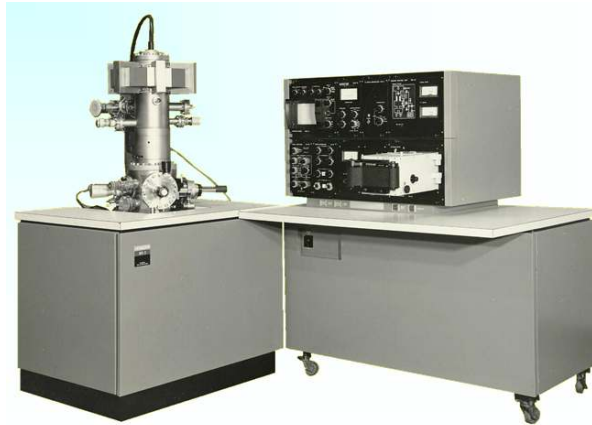
Hitachi's World First Commercial FE-SEM, Model HFS-2 (1972)
