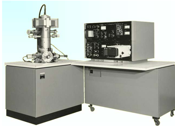
Hitachi's World First Commercial FE-SEM, Model HFS-2 (1972)
