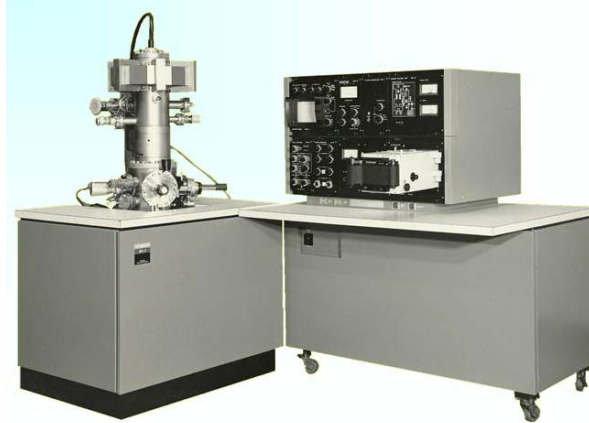
Hitachi's World First Commercial FE-SEM, Model HFS-2 (1972)
