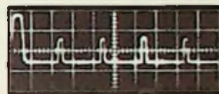
Delayed Sweep display of a pulse chain—with the fourth pulse intensified by trace brightening. This brightened area indicates the delayed sweep start and duration. With both the start and duration adjustable. It is possible to include any portion of the displayed waveform in the brightened area.
