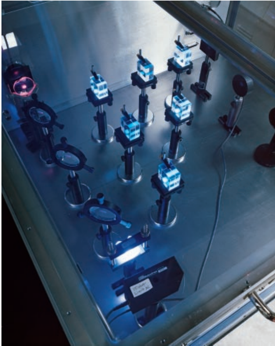
FIGURE 2. Samples of fused silica being irradiated at 193 nm in the Lincoln Laboratory test and evaluation facility for optical materials. Research at this facility is being done to quantify the magnitude of various laser-induced effects on optical materials, and their scaling with laser intensity, pulse count, and geometry of irradiation. The visible fluorescence seen above indicates that the fused-silica materials in this experiment are not fully transparent at 193 nm.
