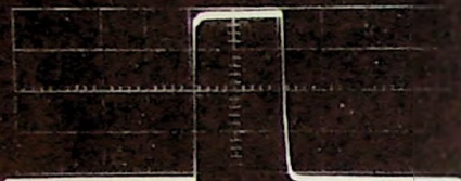
UNRETOUCHED PHOTO OF OUTPUT PULSE, MODEL L2005 (Horizontal scale: 5 \mu sec/cm)
