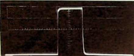
UNRETOUCHED PHOTO OF OUTPUT PULSE, MODEL L2005 (Horizontal scale: 5 \mu sec/cm)
