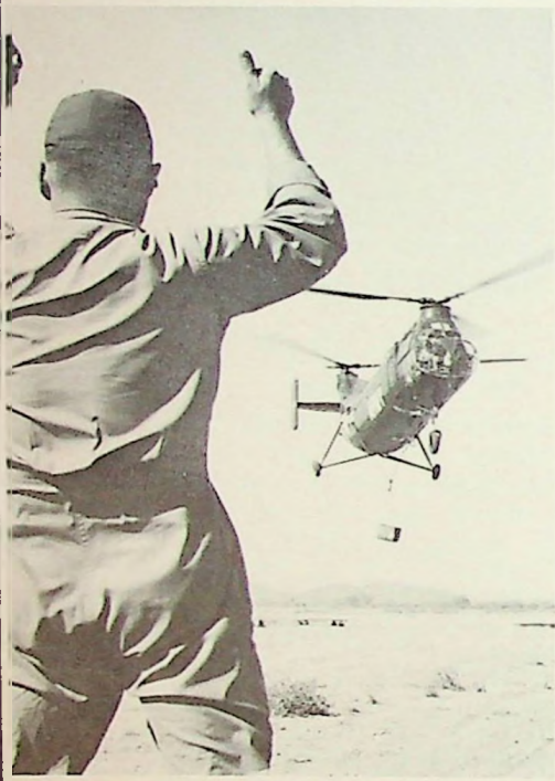
Universal automatic pilot developed for the Army by Sperry Phoenix Co. gets prototype testing in typical Arizona scenery. Six-hundred-pound load swinging beneath Army H21 helicopter provides forces attempting to "upset" control equipment
