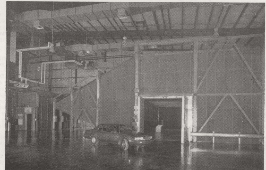
Test Vehicle at Entrance to TEM Cell
