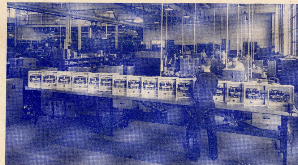
Reversing Starters on test in one of several of the test departments of the Square D Company to be visited on Wednesday afternoon.
