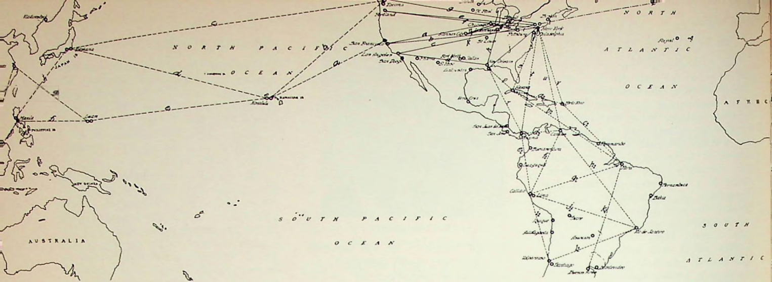
Transpacific, transatlantic, South American, and domestic systems of the Federal Telegraph Co., San Francisco, planned by the company in 1914 with a 100-kw transmitter and operating room in South San Francisco.
