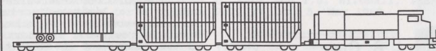
Tags mounted on Railcars, Trailers, and Containers provide train consist information for terminal arrival/ departure notification.
