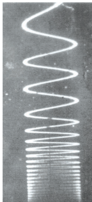
Fig. 12. Fringe signal on dropping one of the two mirrors in an interferometer.
