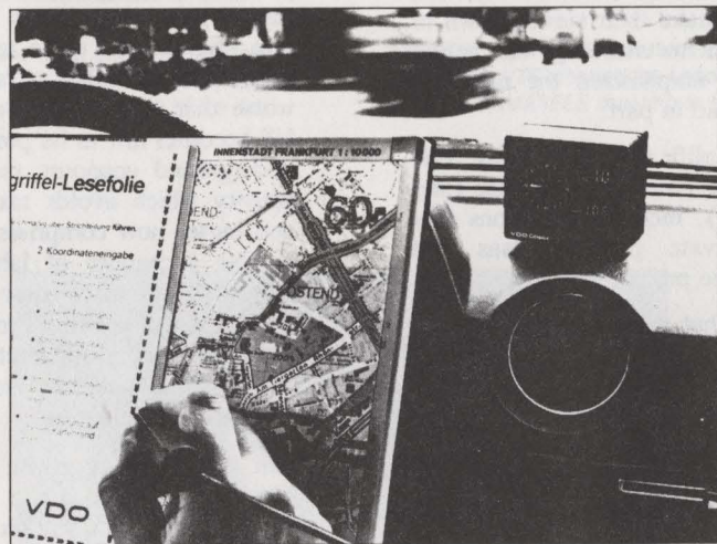
City Pilot Smart Compass Uses Data Picked Up From A Bar-Coded Map By Light Pen and Fed Into A Microcomputer. Distance and Location Information Are Displayed On An LCD.
