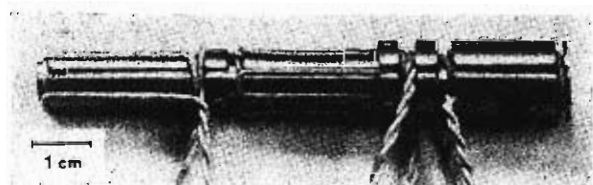
FIG. 4. The magnetic double-deflection and astigmatism corrector. The right-hand winding is the 1st deflector, the left-hand winding is the 2nd deflector, and the center winding is the astigmatism corrector.
