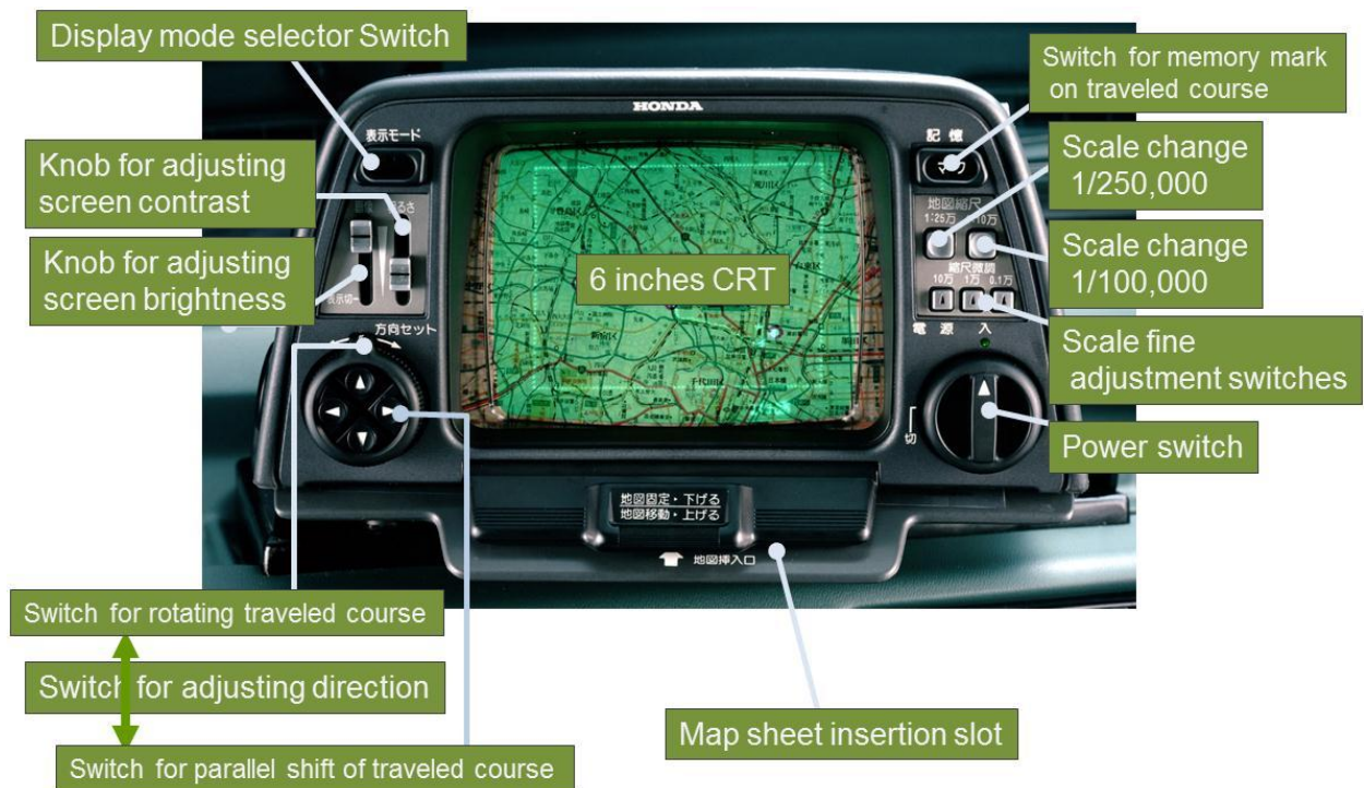
Fig. 5: Switches configuration of display equipment (front view)
