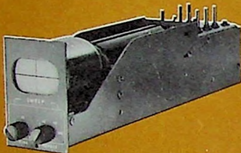
MODEL 260M Plug-in Scope—2" flat faced CRT; frequency response DC to 1 megacycle; sensitivity 0.25 to 2.5 volts rms in. of deflection; input impedance 100K ohms; sweep rates 10 cps to 10 KC; triggered or free running operation.
