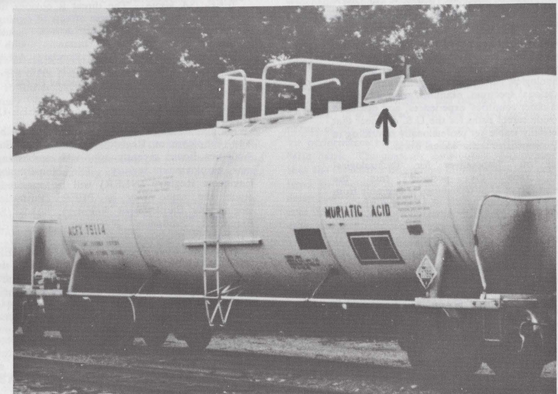
Railroad tank car has Railstar transmitter (see arrow) which can send data on identity, valve positions, temperature and pressure of contents. This transmitter is solar powered but units on trucks could be powered from the truck's power generation system.
