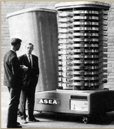
figure 8. An ASEA thyristor test valve (photo courtesy of the IEEE).
