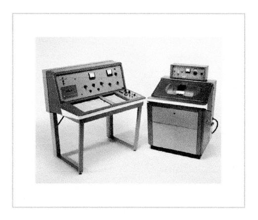
The A-60 was the workhorse NMR instrument for decades as it allowed chemists to determine molecular structures easily and quickly and to follow the progress of chemical reactions. Courtesy Agilent Archives.
