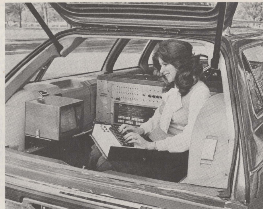
Unique vehicular testbed which permits on-the-road investigation of engine control strategies--the computerized vehicle was developed at GM Research Labs.
