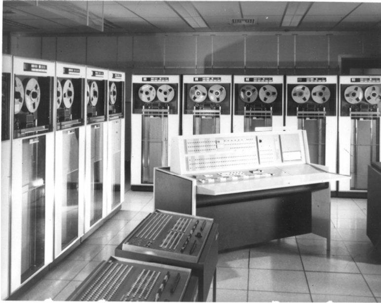
Fig. 3-1. The computer center at Bell Labs in Murray Hill around 1963 consisted of an IBM 7090 computer. Input and output were on magnetic tape. The operator monitored the operation of the computer at a console. [Photo courtesy of Alcatel-Lucent USA Inc. / Bell Labs.]
