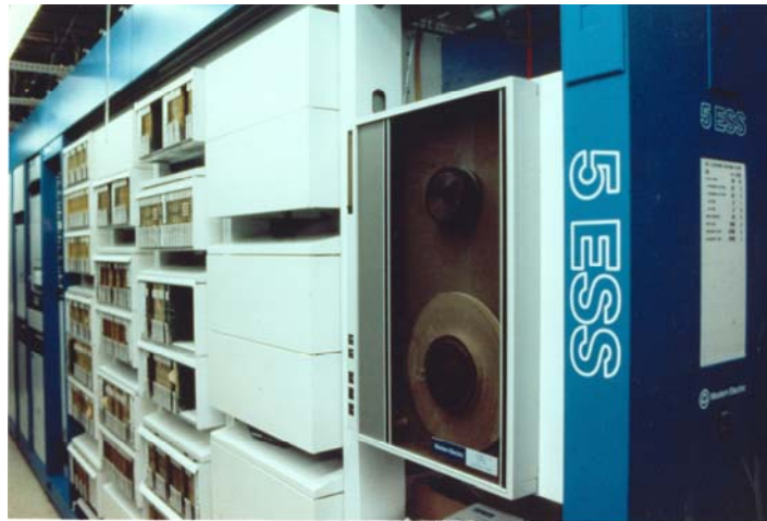
Fig. 5-16. The 5ESS® switching system was manufactured initially by Western Electric, with its initial installation in 1982, and later by Lucent Technologies. It is an all-digital switching system with time-slot interexchange. [Photo courtesy of Alcatel-Lucent USA Inc. / Bell Labs.]
