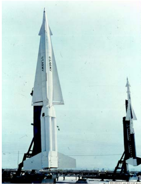
Fig. 5-20. Bell Labs designed the guidance system for the series of Nike anti-aircraft missile systems. The Nike Hercules missile is on the left; the Nike Ajax is on the right in this photo from 1960. The Nike Zeus was aimed against ballistic missiles, but was not implemented. [Photo courtesy of Alcatel-Lucent USA Inc. / Bell Labs.]
