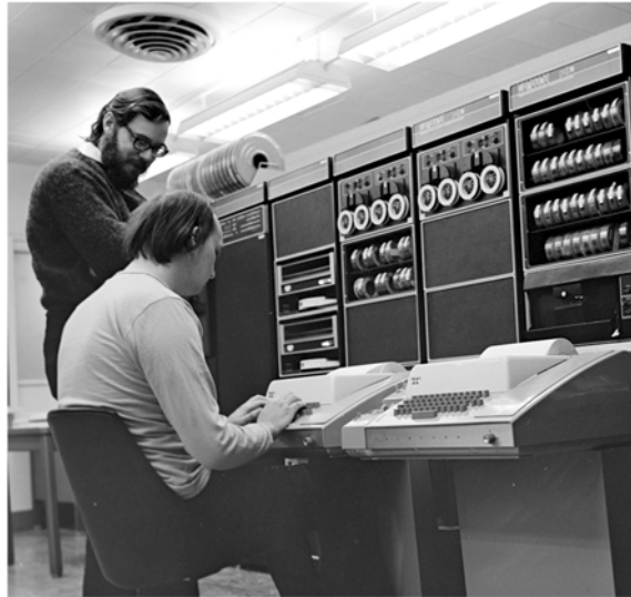
Fig. 5-7. Ken Thompson (sitting) and Dennis Ritchie (standing) invented the Unix operating system in the early 1970s at Bell Labs. They are shown in this 1972 photograph at a terminal connected to a Digital Equipment Corporation PDP-11 computer. Variations of their Unix system are today the basis for many computer and tablet systems. [Photo courtesy of Alcatel-Lucent USA Inc. / Bell Labs.]
