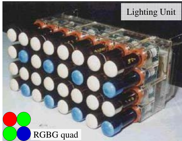
Design of pixel RGBG quad was first application for display in practical use.
