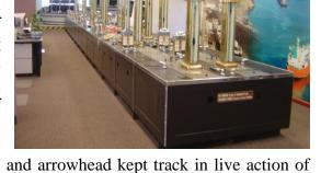
Tall barometer-like encased glass tubes with a scale and arrowhead kept track in live action of the level of water in each of the six lock chambers (two rows of three locks each to make up the set of locks).
