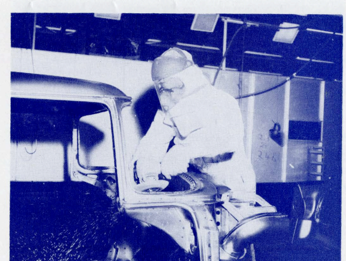
Discing and grinding operations performed on Ford bodies at the Ford-San Jose Assembly Plant. W. J. Holden
