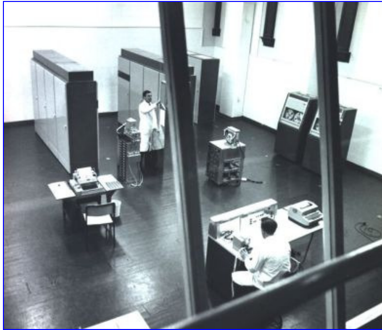
Fig. 9. The Cambridge Titan computer, prototype of the Atlas 2, photographed from the viewing gallery.
