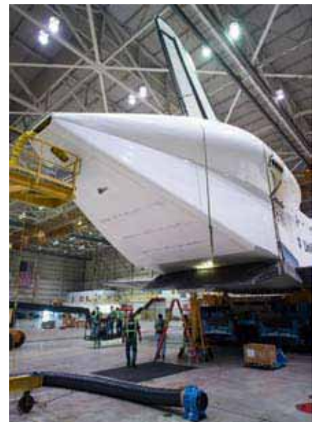
Workers prepare to remove the tail cone off of the space shuttle Endeavour in a hangar at Los Angeles International Airport, September 24, 2012. Photo (Credit: NASA/Bill Ingalls)
