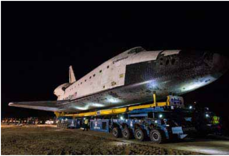
The space shuttle Endeavour, sitting on the Overland Transporter and the Self-Propelled Modular Transporter, moves out of the Los Angeles International Airport and onto the streets of Los Angeles. (Photo Credit: NASA/Carla Cioffi)
