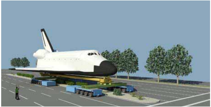
An artist rendering of the Space Shuttle Orbiter on the Overland Transporter with the Self-propelled Modular Transporters (SPMT). (Photo Credit: California Science Center)
