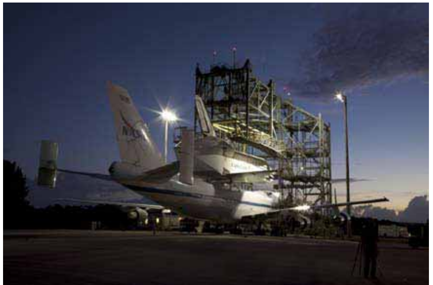
As the sun rises at the Shuttle Landing Facility at NASA's Kennedy Space Center in Florida, preparations are under way to back NASA's Shuttle Carrier Aircraft, or SCA, away from the Mate-Demate device. Space shuttle Endeavour has been fitted with an aerodynamic tailcone and secured atop the aircraft for its ferry flight. (Photo credit: NASA/Frankie Martin)
