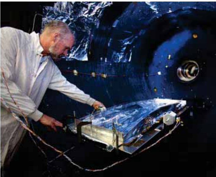
Figure 5. Northrop Grumman Lead Venting Analyst Dan McGregor with a sunshield test article as it is placed in the vacuum chamber at Aerospace Systems' test facility in Redondo Beach, CA. Image Credit: Northrop Grumman Aerospace Systems
