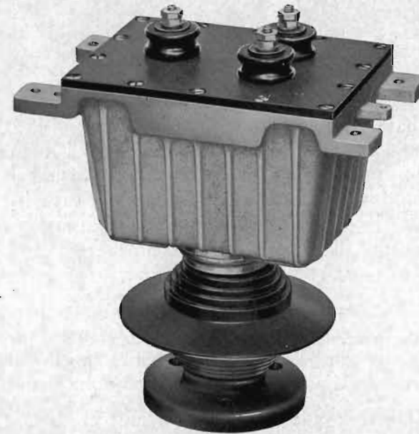
Antenna Shortening Condenser of smaller capacity for small equipments, maximum amperes 8, maximum voltage 30,000, capacity .0006 and .0008, $45.00. Without insulated base, $35.00
