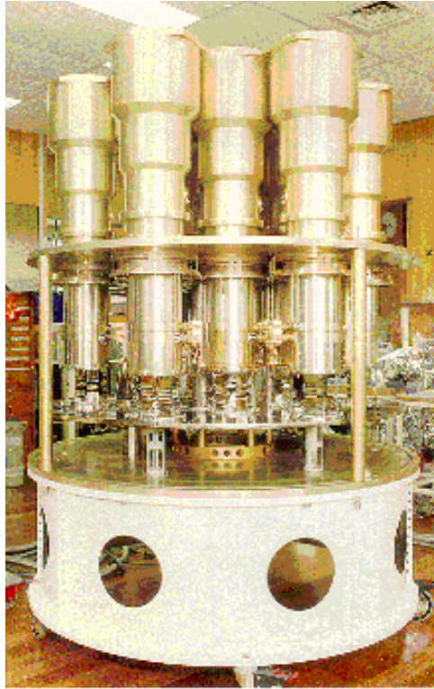
Figure 24 - The Parkes 21cm Multibeam Receiver
