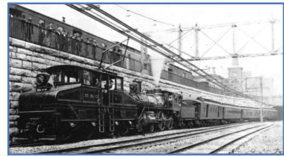
figure 11. Electric locomotives were placed ahead of the steam engine on northbound passenger trains as shown in this view that appears to show the inaugural run on 1 July 1895 (source: A Guide to Trains , Fog City Press, 2002, p. 55).
