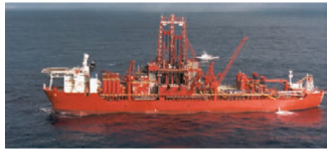
Fifth-generation DP drillship, the Seadrill West Navigator, drilling offshore Norway in the summer of 2000.
