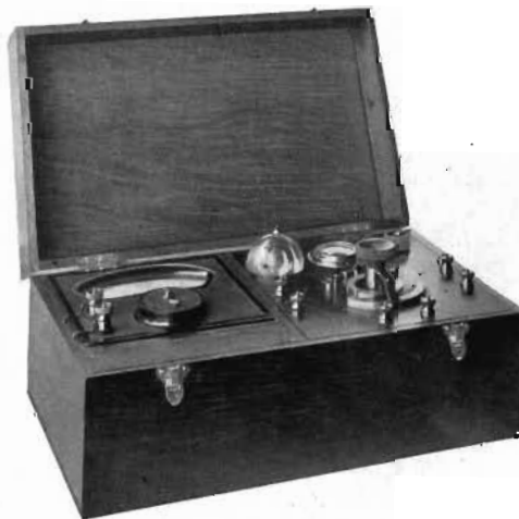
High-Resistance Voltmeter, low-range, combined D.C. and A.C. pattern. Ranges: 0-1, 0-10, 0-100, 0-1,000 volts D.C.; and 0-2.5, 0-25, and 0-250 volts A.C.
