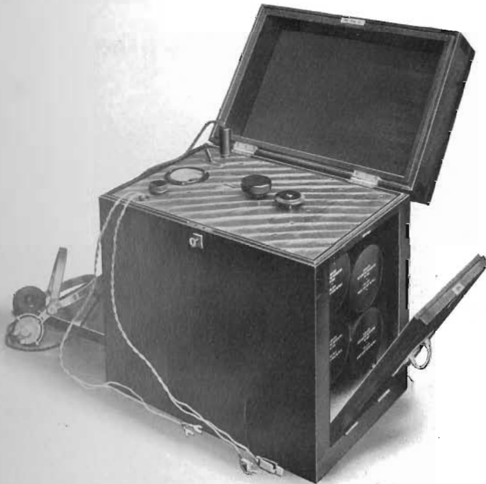
Long-range Heterodyne Wavemeter, with plug-in inductances (50-20,000 metres)
