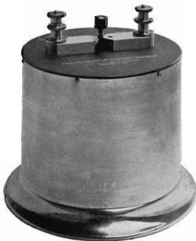
Laboratory Fixed-Capacity Standard Condenser in polished brass case
