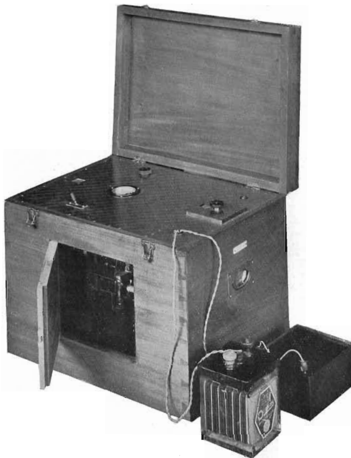
Short-wave Heterodyne Wavemeter, 5-70 metres
