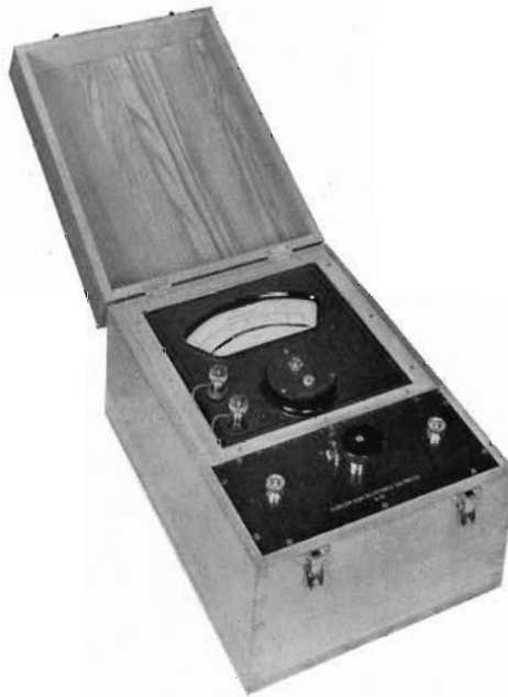
High-Resistance Voltmeter, low-range D.C. pattern. Three ranges: 0-12, 0-120, and 0-360 volts
