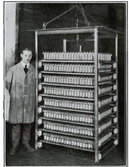
Interior arrangement of one unit of oil-immersed Paper Dielectric Smoothing Condenser
