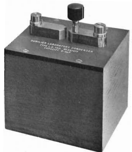
Laboratory Fixed-Capacity Standard Condenser in polished wood case
