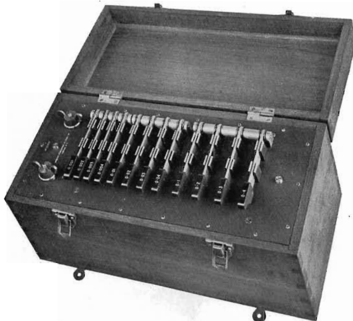
Laboratory Adjustable-Capacity Standard Condenser, knife-switch type. Max. capacity 1.11 microfarads. Condenser Type LS12/1.11L/KS12
