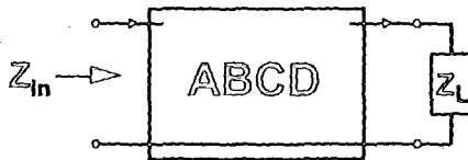
Figure 2.6.6. Input impedance of a two-port with arbitrary load impedance.
