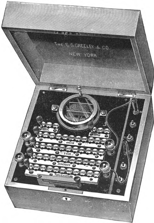
FIG. 172. Wheatstone Bridge Apparatus, with Galvanometer and Battery.
