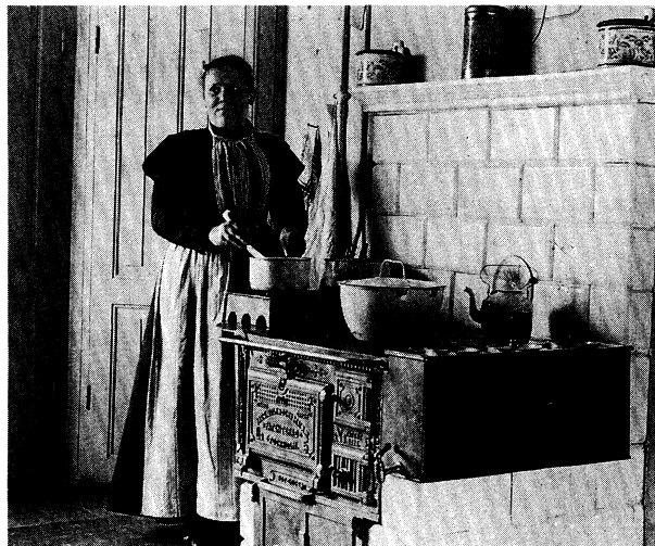
Figure 3. Gas cooker on top of a traditional wood stove. (Photo from the turn of the century)
