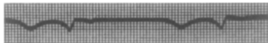
Fig. 4.—Same condition as in Fig. 1, with the exception that an extra resistance of 100,000 ohms has been introduced into the galvanometer circuit.
