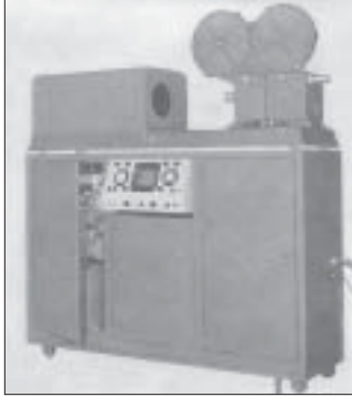
Before the advent of videotape recording, most television originated from motion picture film. The television film "chain" shown here included a 16-mm projector and a Vidicon television camera. Photo courtesy of General Electric
