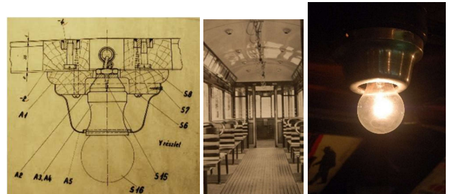
Fig. 8.: Tungsten filament lampholder's cross section from the 30-ies [2] – lamps in a tram [8] – lamp in the URM
